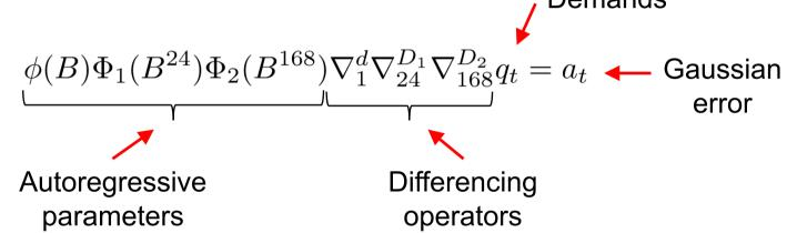
**Challenge:** How do we estimate the unobserved demands and VARIMA model parameters using limited observed hydraulics?
